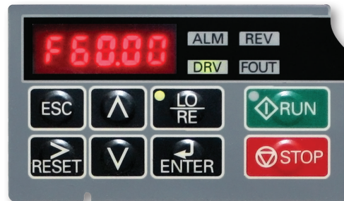
5 digit keypad with LED status display
