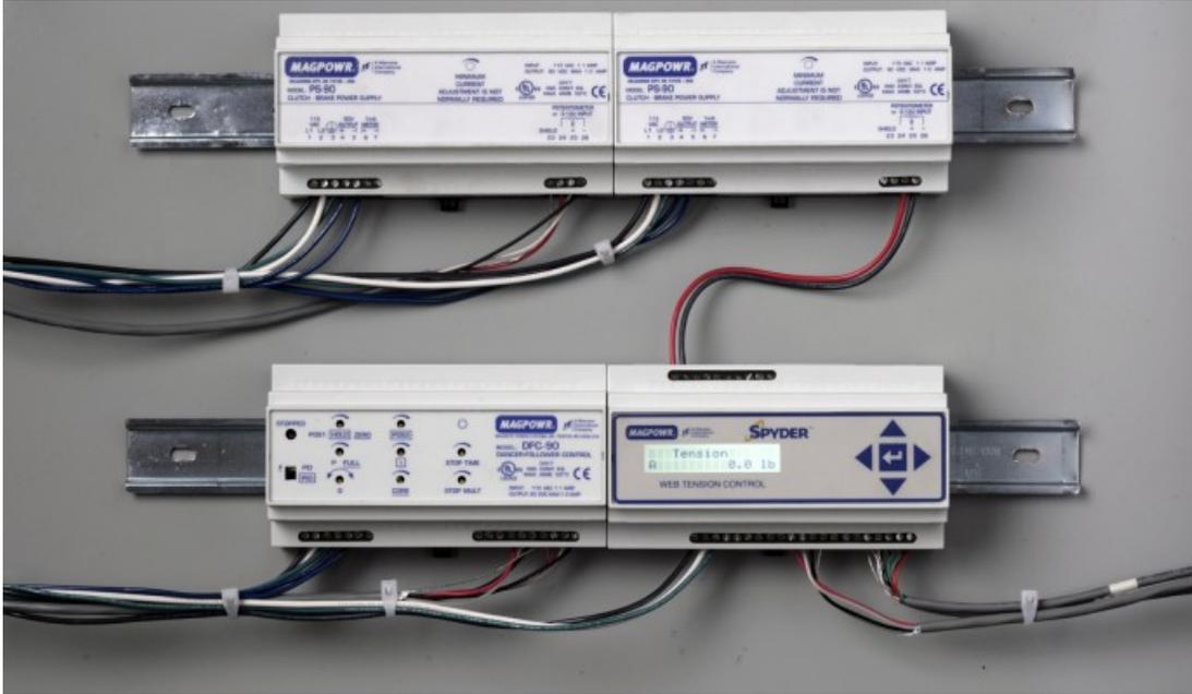
Complete control is the goal of any operation utilizing brakes and clutches. MAGPOWR's PS-24 & PS-90 Power Supplies provide a small amount of reverse current circuitry as a standard feature to minimize the drag torque of a clutch/brake, allowing greater controllability in the lowest torque range.
